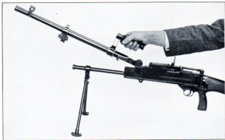
FIG. 9. The Barrel Change—Second Stage.
