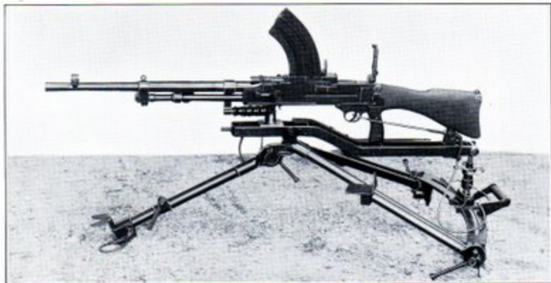
FIG. 12. The Vickers-Berthier on Tripod Mounting—Low Position.
