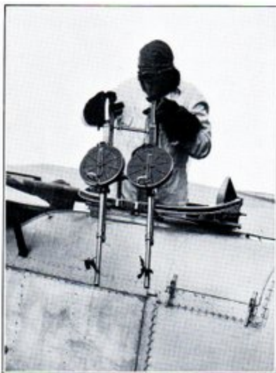
FIG. 16. Two Vickers-Berthier Aircraft (observer's) automatic guns on twin mounting.
