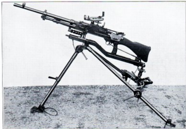
FIG. 13. The Vickers-Berthier in position for indirect firing. Note the dial sight and clinometer.
