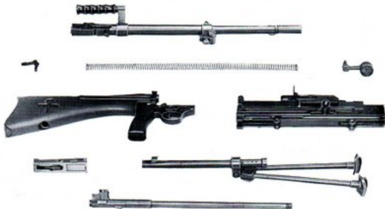
FIG. 7. The Vickers-Berthier dismounted to show the main parts.
