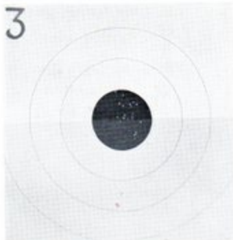
FIG. 5. Automatic Accuracy Test of the Vickers-Berthier Light Machine Gun. The target (12 in. — 30.4 cm. bull) after firing. Range, 100 yards (91 metres). This series was fired immediately after the 1,000 round series shown in Fig. 4 with the same gun and barrel.
